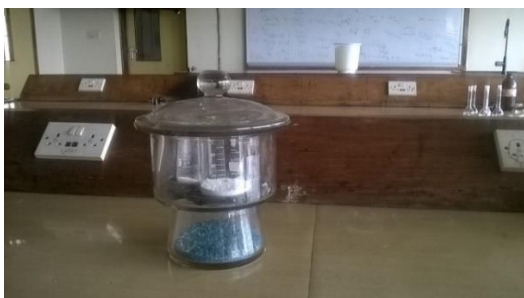
Photo: 7 cooling in a desiccator
