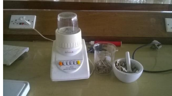
Photo: 2 Blender, mortar and pestle for grinding
