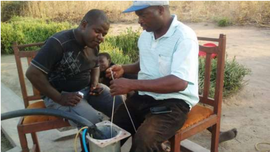
Figure 3: Technicians Taking a Reading for Water Level during Pumping Test
