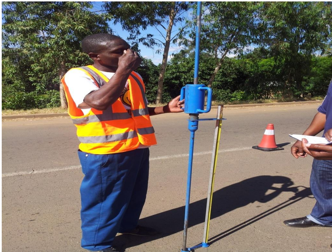
Figure 3.4: DCP Test on Mugabe Highway
